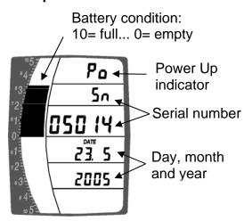
The Startup Screen shows the serial number, the battery condition and the date. The analog scale on the left shows the battery charge.
